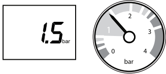
Fig.47 Restore water pressure
